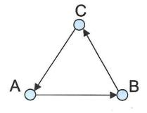
$$D = \begin{pmatrix} 0 & 1 & 0 \\ 0 & 0 & 1 \\ 1 & 0 & 0 \end{pmatrix} \qquad \begin{array}{c} NOT \\ Symmetric \end{array} \qquad D = \begin{pmatrix} 0 & 1 & 1 \\ 0 & 0 & 1 \\ 0 & 0 & 0 \end{pmatrix}$$
